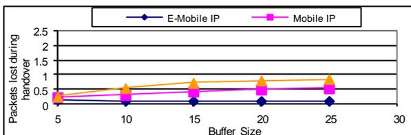
Fig. 5. Packet loss vs buffer size.
